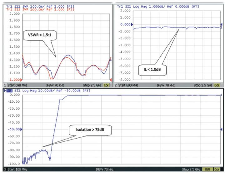
Better than 75dB of Isolation. Rejects Signals from: UHF, VHF and PTC broadcast bands. Filter is designed specifically for locomotive applications.
