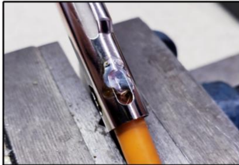
Step 6: Bridge the bulging braids to the connector with solder. Do not solder all four openings, only two opposite windows to reduce risk of damage to the cable. There should be enough solder to hold the braids onto the connector.
