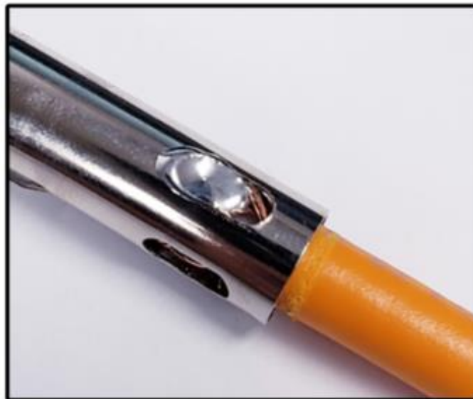
Step 6: Bridge the bulging braids to the connector with solder. Do not solder all four openings, only two opposite windows to reduce risk of damage to the cable. There should be enough solder to hold the braids onto the connector.
