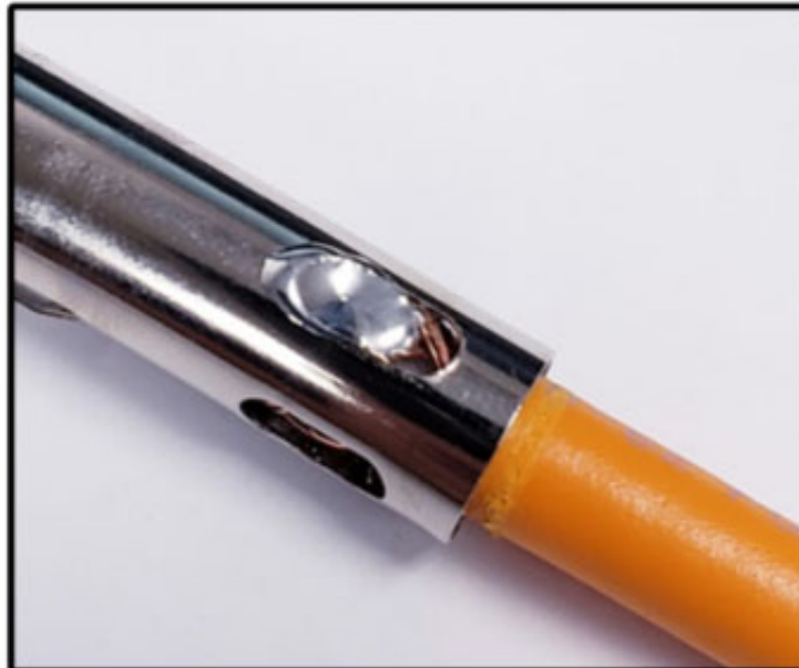
Step 6: Bridge the bulging braids to the connector with solder. Do not solder all four openings, only two opposite windows to reduce risk of damage to the cable. There should be enough solder to hold the braids onto the connector.
