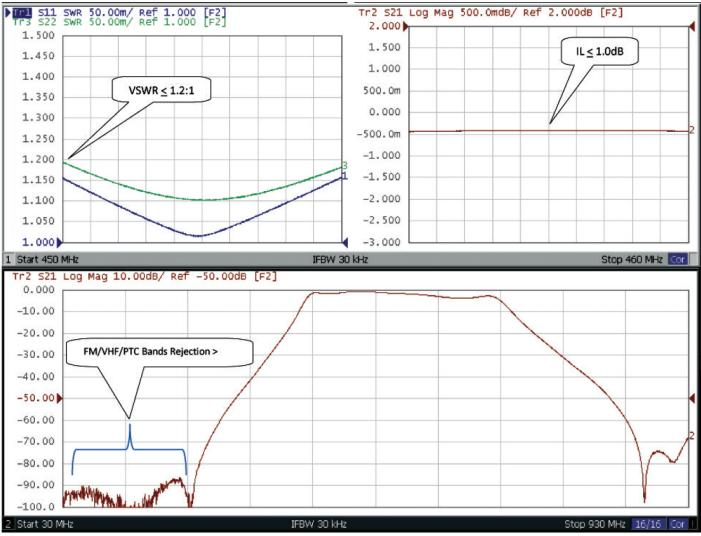
Rejects Unwated RF Signals from: FM/VHF/PTC Bands Filter is designed specifically for locomotive applications
